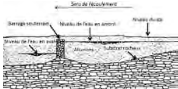
Figure 1 : Schéma d'un barrage souterrain (Adapté de https://www.oas.org/dsd/publications/Unit/oea59e/ch34.htm )
